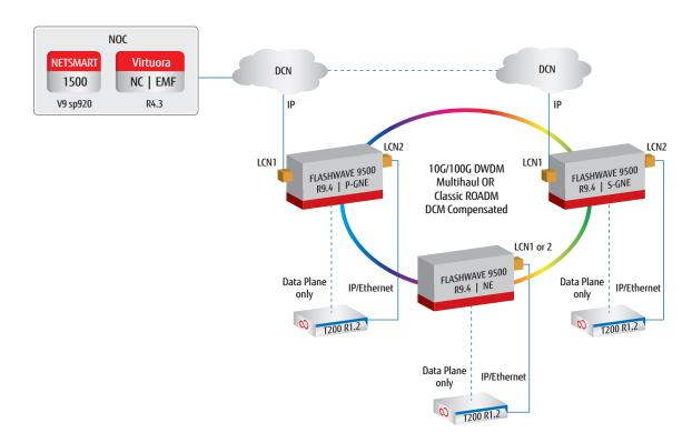
Cost-effective capacity expansion with the 1FINITY T200 Transport blade
